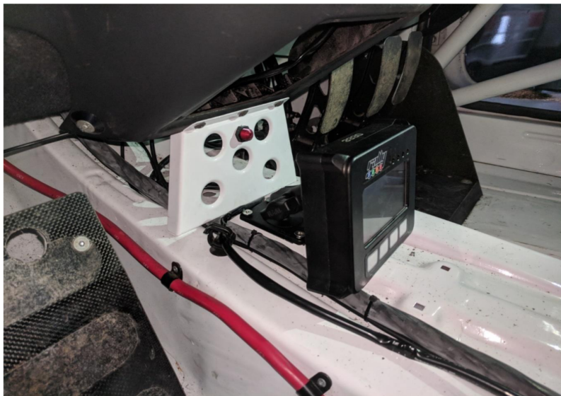
The RallySafe unit then mounts to the 25mm rubber ball mount (connected through the RallySafe connector).
