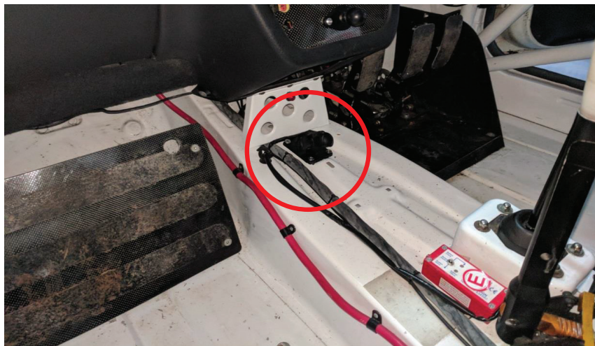
Figure 1. 25 mm rubber ball securely attached to the tunnel.
