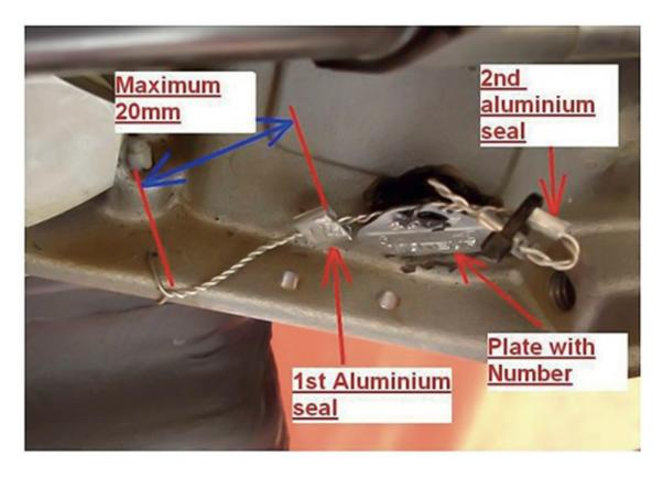
Note: Car will not be allowed to enter scrutineering if sealing wires are not installed beforehand!
